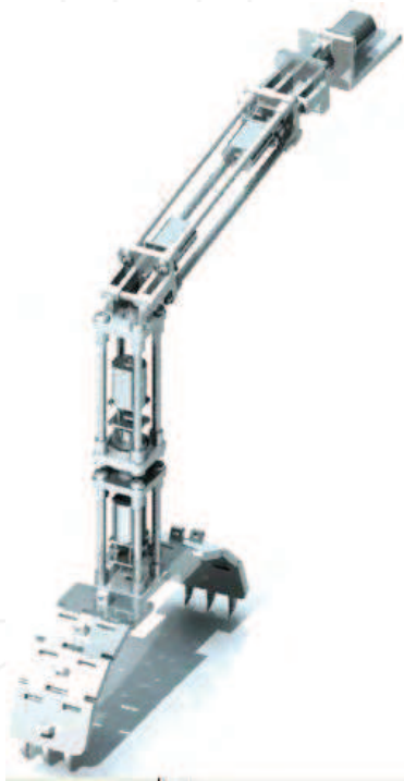
Fig. 2. Kinematic configuration of a leg
