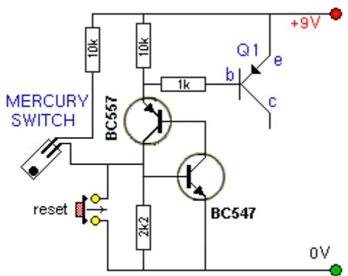
MERCURY TILT SWITCH DETECTION
