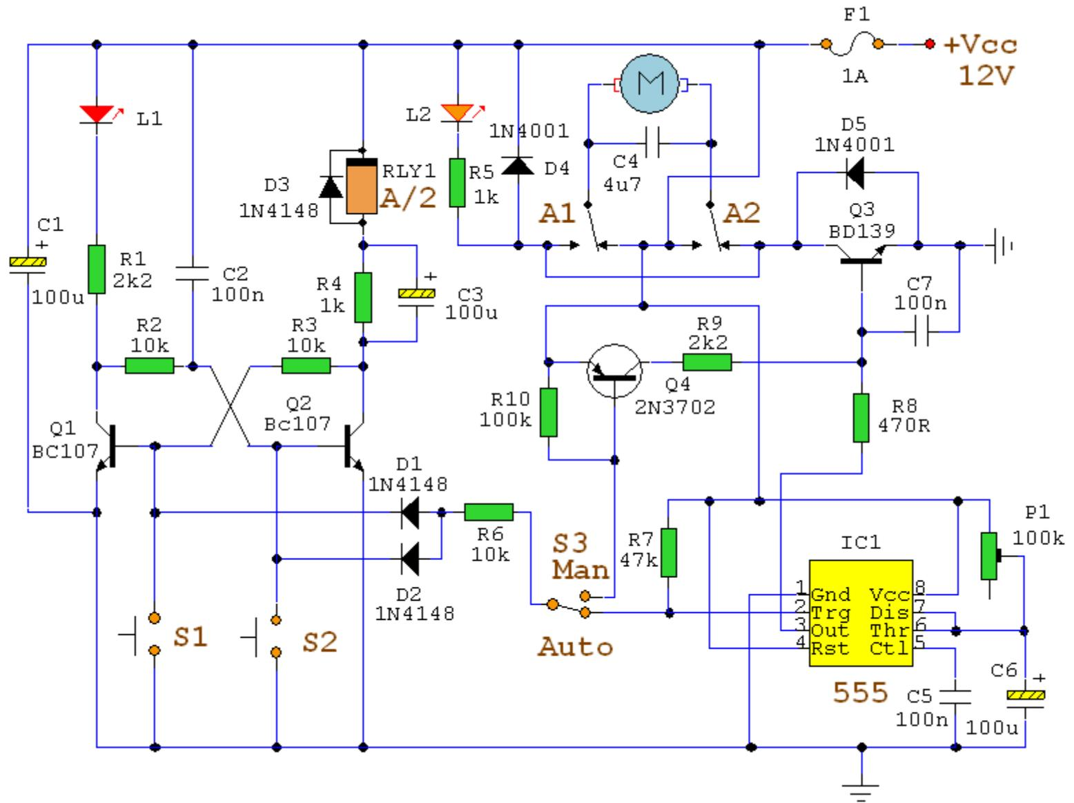
This circuit uses a mixture of transistors, an IC and a relay and is used to automatically open and close a pair of curtains. Using switch S3 also allows manual control, allowing curtains to be left only partially open or closed. The circuit controls a motor that is attached to a simple pulley mechanism, to move the curtains.
