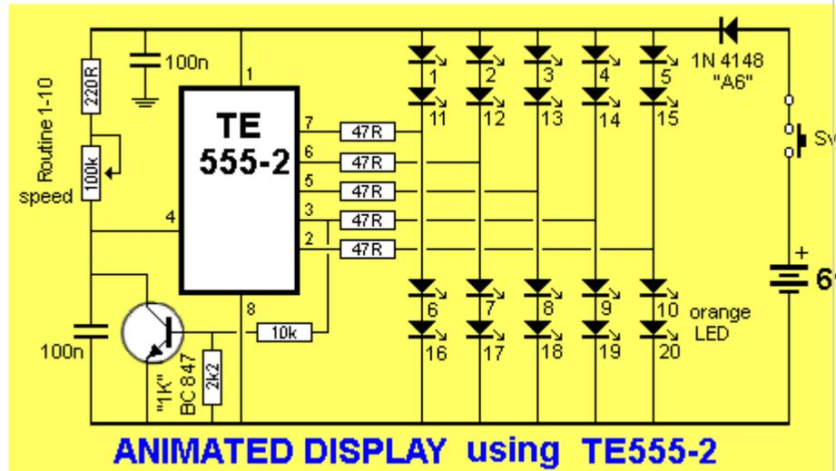
A kit of components (matrix board, PC board for LEDs, surface-mount resistors, capacitors, transistor, diode, switch, cells, battery holder, pot and 20 yellow LEDs with TE555-2 chip) is available for \$15.00 plus \$5.00 postage. Click the link above and you will be sent an email with the costs. This is an ideal project you get you into surface-mount technology and you can add it to a model layout or build it into a Lego brick for a junior member.
