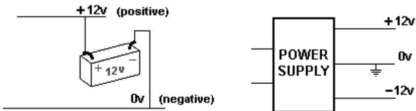
Sometimes you will see a circuit as shown in the **first diagram** with 12v or +12v on the top rail and 0v or a negative sign or the word "negative" on the bottom rail. In **this case** the word negative means earth or "chassis of a car" and we commonly refer to this as "negative earth" or "negative chassis."
