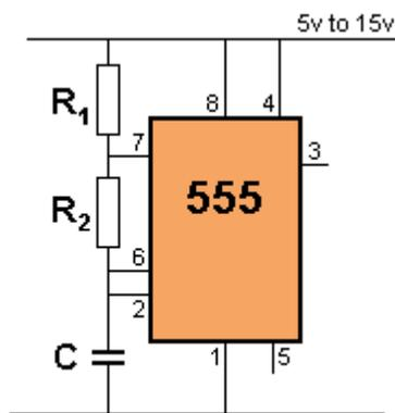
The capacitor C charges via R1 and R2 and when the voltage on the capacitor reaches  $\frac{2}{3}$  of the supply, pin 6 detects this and pin 7 connects to 0v. The capacitor discharges through R2 until its voltage is  $\frac{1}{3}$  of the supply and pin 2 detects this and turns off pin 7 to repeat the cycle.
