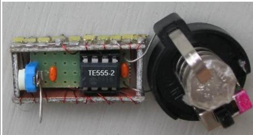
The project has two 10-LED displays. One on the front and one on the back
