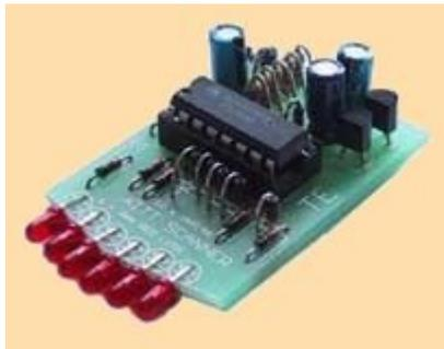
Here is a simple Knight Rider circuit using resistors to drive the LEDs. This circuit consumes 22mA while only delivering 7mA to each LED. The outputs are "fighting" each other via the 100R resistors (except outputs Q0 and Q5).
