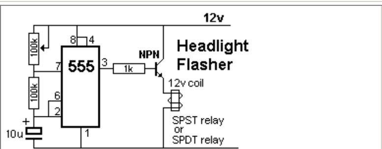
Here is a simpler circuit. It will need testing and adjusting to suit the relay you will be using:
