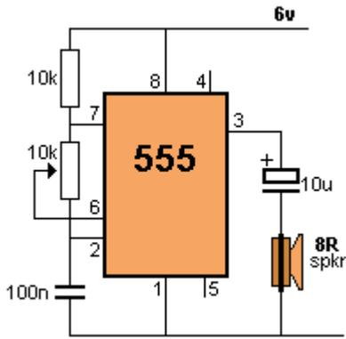
4. Do not draw 555 circuits as shown in the following diagram. Keep to a standard layout so the circuit is easy to follow.
