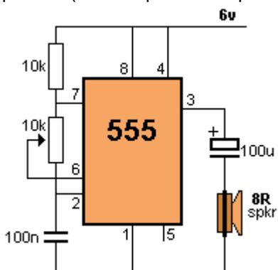
3. The reset pin (pin 4) is internally tied HIGH via approx 100k but it should not be left floating as stray pulses may reset the chip.
