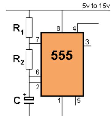
If the capacitor is replaced with an electrolytic, the frequency of oscillation will reduce. When the frequency is less than 1Hz, the oscillator circuit is called a timer or "delay circuit." The 555 will produce delays as long as 30 minutes but with long delays, the timing is not accurate.
