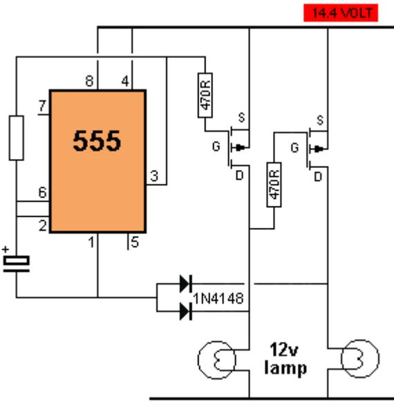
The 555 circuit uses two diodes to connect the chip to the negative rail and this allows the components to be fitted between the "high side" of the lamps and the "power switch."
