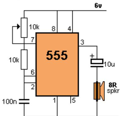
2. The impedance of the 100u electrolytic will allow a very high current to flow and the chip will get very hot. Use 10u maximum when using 8R speaker. (The temp of the chip will depend on the frequency of the circuit.)
