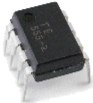
This circuit uses the latest [TE555-2](#) ANIMATED DISPLAY CONTROLLER chip from Talking Electronics. This 8-pin chip is available for \$2.50 and produces 7 different animations on a 10 LED display. The animations are selected by the position of a 100k pot and when the animation is showing, the pot can be adjusted to increase the speed of the animation. "Position 10" on the pot cycles through the 7 animations.
